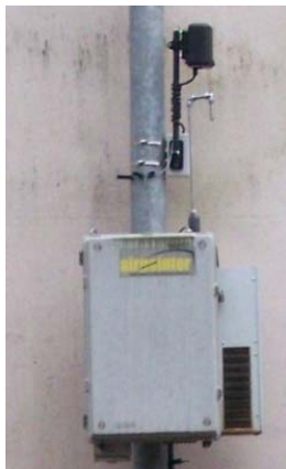
Plate 3. Close up of the Airpointer and MOVA sensor
