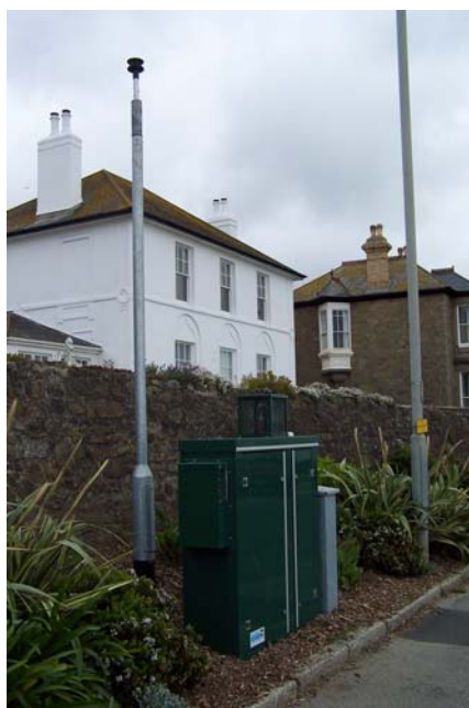
Plate 1. The sulphur dioxide monitor and anemometer at Chyandour Cliff, Penzance.
